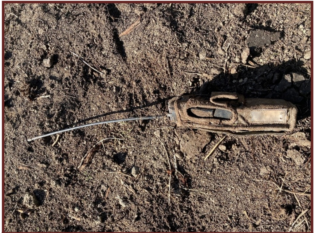
Figure 2: The swamper’s radio, found at the accident site still inside the holster. The radio fell off when the pack was removed during extraction from the juniper.
